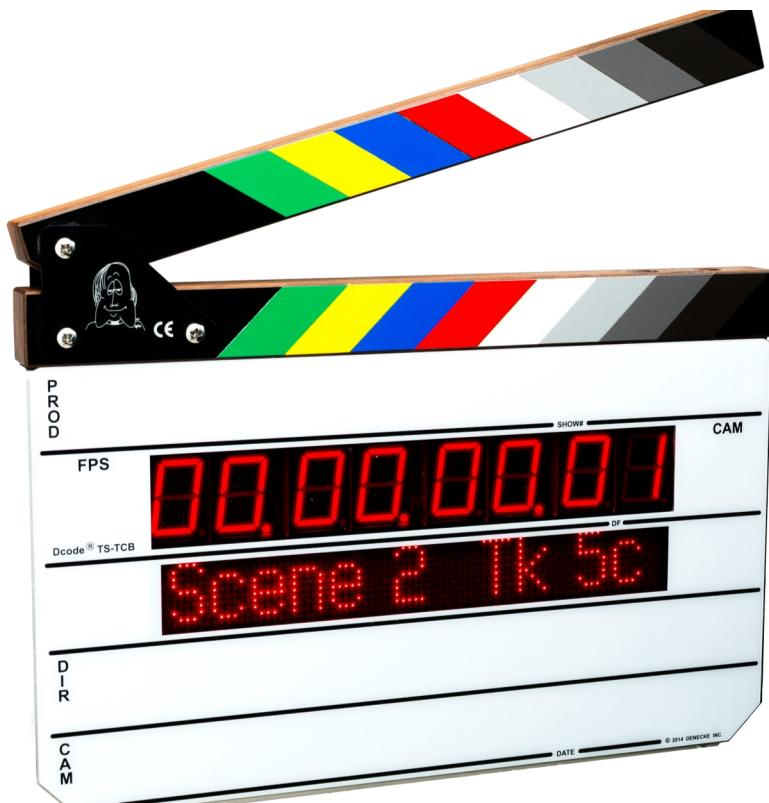
The Denecke TS-TCB combines the convenience and functionality of a traditional solid hardware timecode slate with accurate RF-locked readout, transmission of stick closing timecode, and a second ultra-bright LED dot matrix display to mirror metadata from iOS applications. That means that production teams can use a real hardware slate with two-way network communication enabled by Timecode Buddy wireless protocols.
